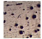
Pearlitic Chill rolls are essentially an indefinite chill-type material. The **microstructure** constitutes nodular graphite and carbides in a pearlitic matrix. The resistance to fire-cracking is best when
