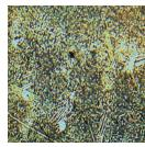
The Alloyed Steel Base microstructure consists of ferrite, pearlite and even some bainite for the higher carbon grades. These materials have no fall-off in hardness with increasing depth. This material has
