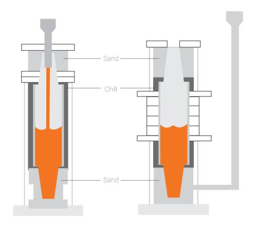
The Static Casting process is used to cast the whole roll in one go so the chemical properties are the same throughout the roll. By employing cooling speed and heat treatment techniques, we are able to manipulate the performance of the roll neck and shell to meet specific requirements. Our static casting process is
