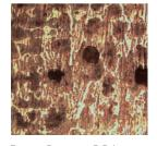
Deep Groove SG has nodular graphite. This material has superior wear resistance at high depth ideal for large sections with deep grooves or seamless tubes.
