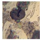
The microstructure of Ferritic Bainite SG ranges from mostly pearlitic to bainitic with graphite nodules that are surrounded by a layer of ferrite giving a characteristic "bull's eye" effect. No signifi-
