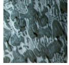
Our standard ICDP made specifically for hot strip mills has a microstructure that includes M3C type eutectic carbides and free graphite embedded in a tempered bainitic martensitic matrix, providing
