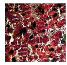
Bainitic Acicular SG has nodular graphite & carbides in an acicular (needle-like) bainitic matrix with increased carbide content & some martensite. This material has superior wear resistance & an excellent
