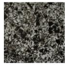
The Graphitic Steel consists of a controlled amount of fine flake graphite particles are dispersed throughout the structure. It has improved the fire-crack resistance as the free graphite reduces the
