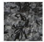
The microstructure of Indefinite Chilled Cast Irons has a carbide-rich yet tough material. The presence of flake graphite enhances chipping resistance and fire-cracking resistance, making Indefi
