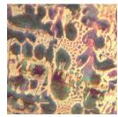
The microstructure of DPIC has a gradual transition from a carbide-rich surface containing a small amount of graphite to a grey core. The surface is intermediate between white & grey iron, with the
