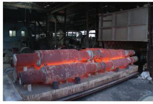
Our company has advanced domestic heat treatment furnaces that are equipped with natural gas-fired units and fans, which improve furnace atmosphere circulation. These furnaces are necessary to address the residual stress caused by heat and structural stress in cast iron rolls. Residual stress
